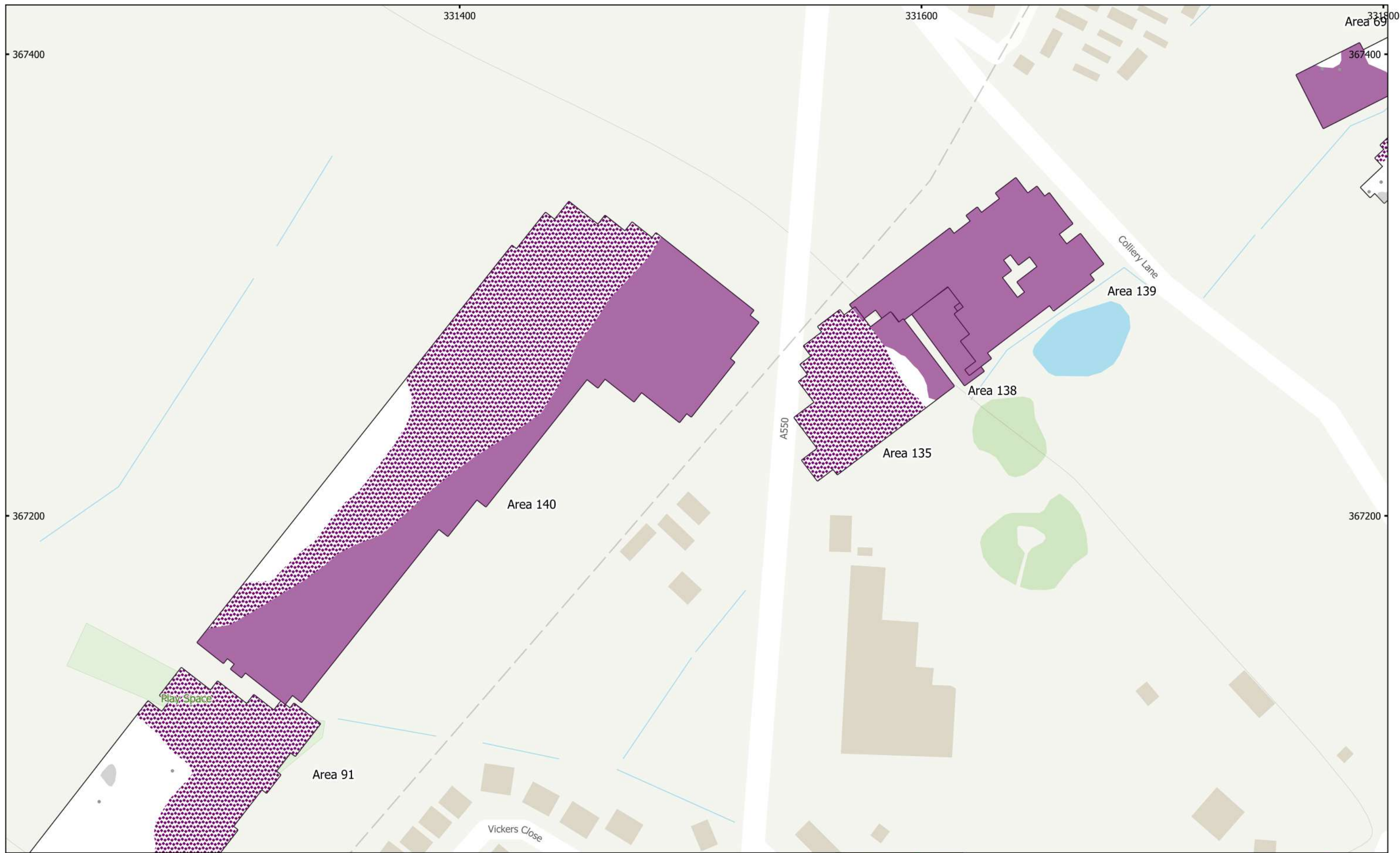
MSSJ1172 - HyNet CO2 Pipeline Figure 115 - Magnetic Interpretation (Areas 68, 69, 91, 135, 138, 139 & 140) 1:1,500 @ A3 Copyright Magnitude Surveys Ltd 2022 Contains Ordnance Survey data © Crown Copyright and database right 2022
