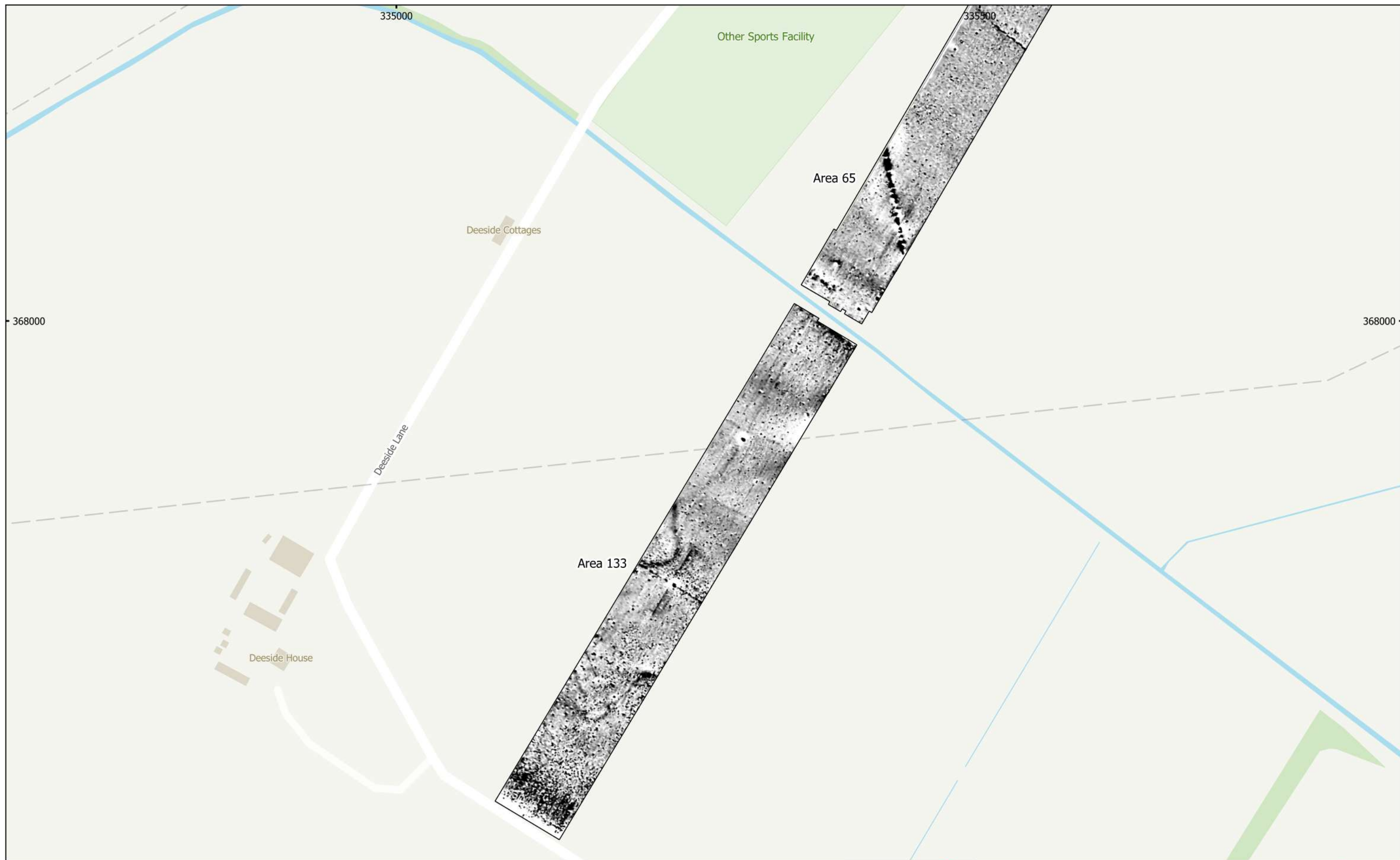
MSSJ1172 - HyNet CO2 Pipeline Figure 28 - Magnetic Total Field (Lower Sensor) (Overview) (Areas 133 & 65) 1:3,000 @ A3 Copyright Magnitude Surveys Ltd 2022 Contains Ordnance Survey data © Crown Copyright and database right 2022
