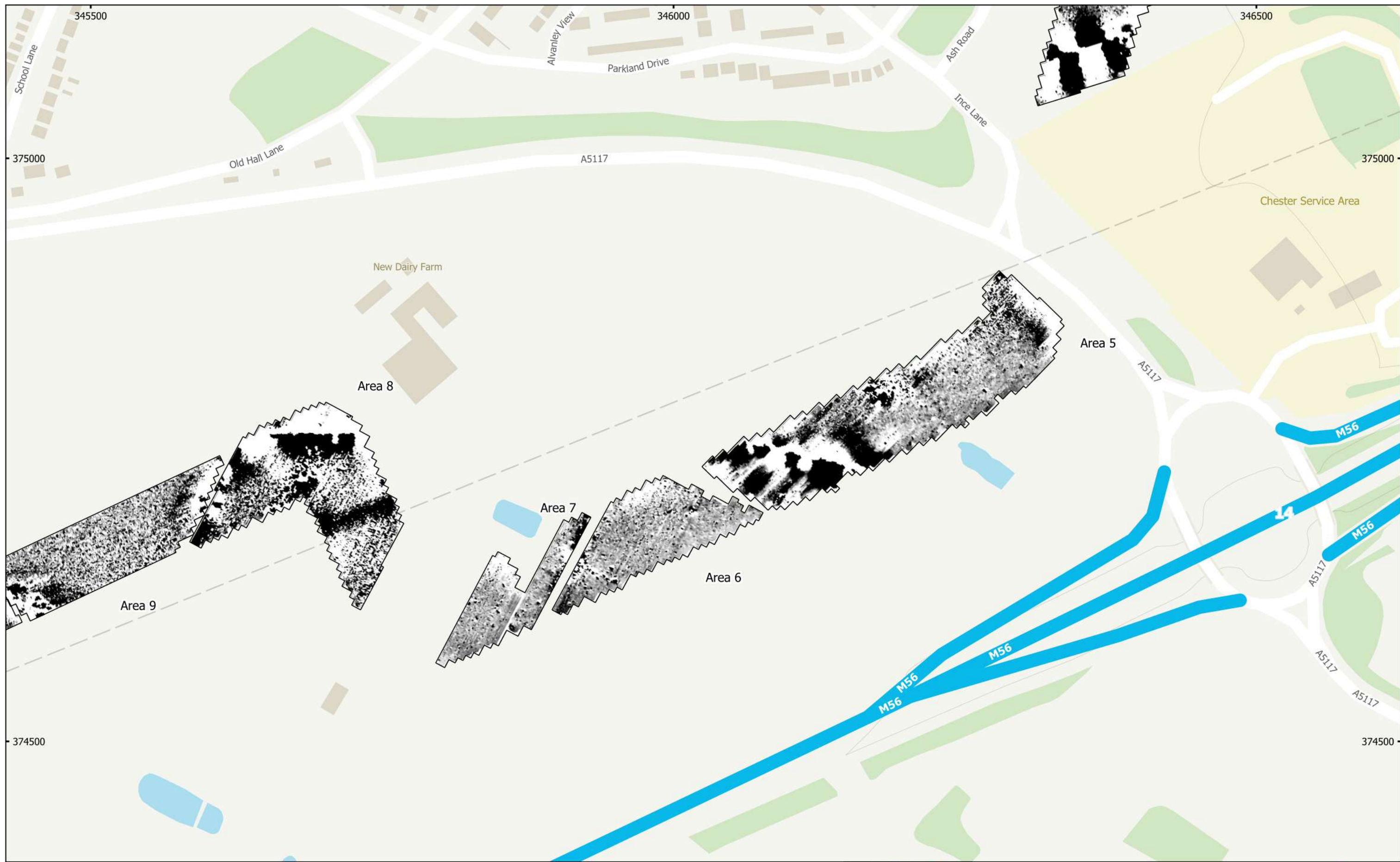
MSSJ1172 - HyNet CO2 Pipeline Figure 54 - Magnetic Total Field (Lower Sensor) (Overview) (Areas 9, 8, 7, 6, & 5) 1:3,000 @ A3 Copyright Magnitude Surveys Ltd 2022 Contains Ordnance Survey data © Crown Copyright and database right 2022
