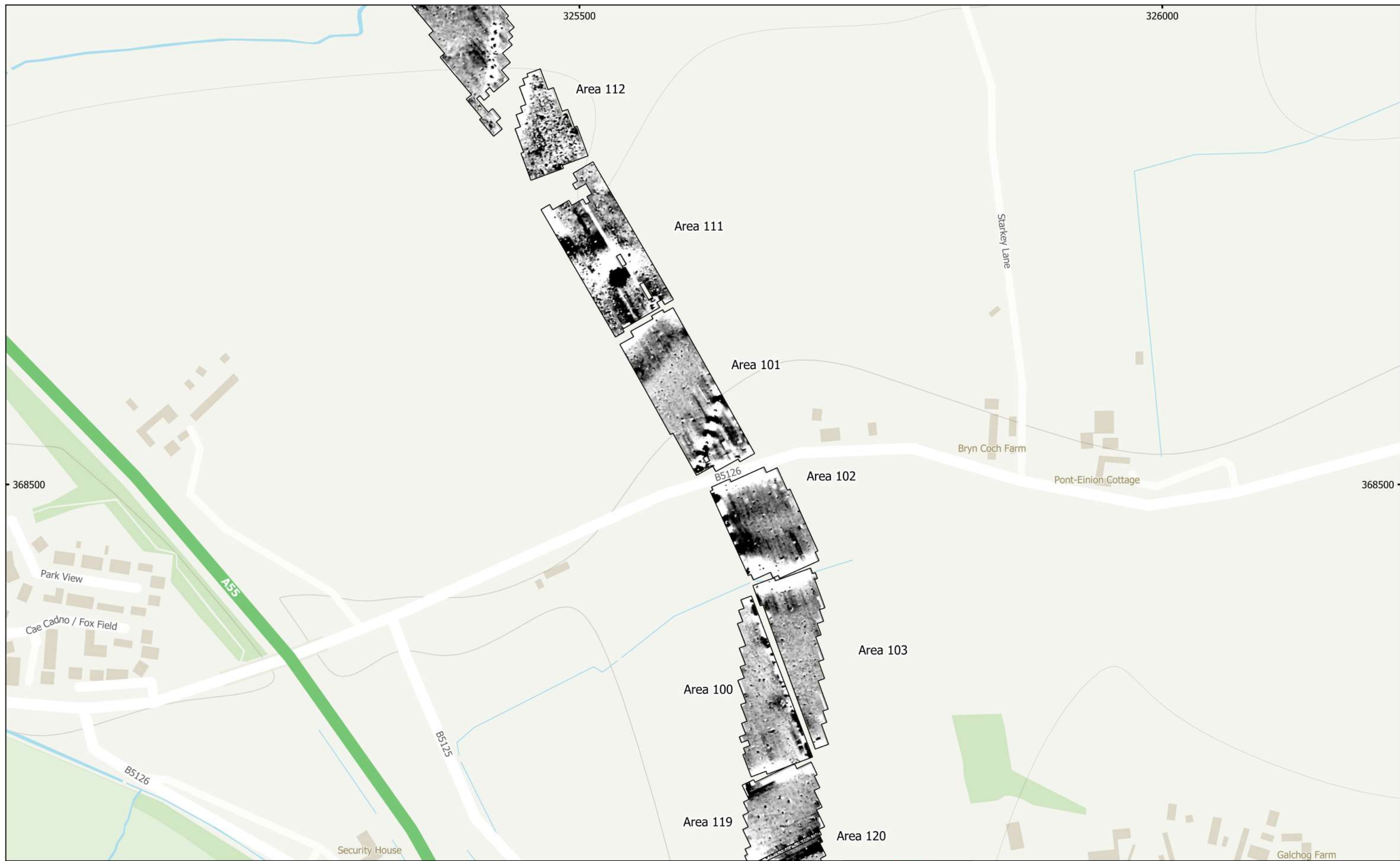
MSSJ1172 - HyNet CO2 Pipeline Figure 10 - Magnetic Total Field (Lower Sensor) (Overview) (Areas 112, 111, 101, 102, 103, 100, 119, & 120) 1:3,000 @ A3 Copyright Magnitude Surveys Ltd 2022 Contains Ordnance Survey data © Crown Copyright and database right 2022
