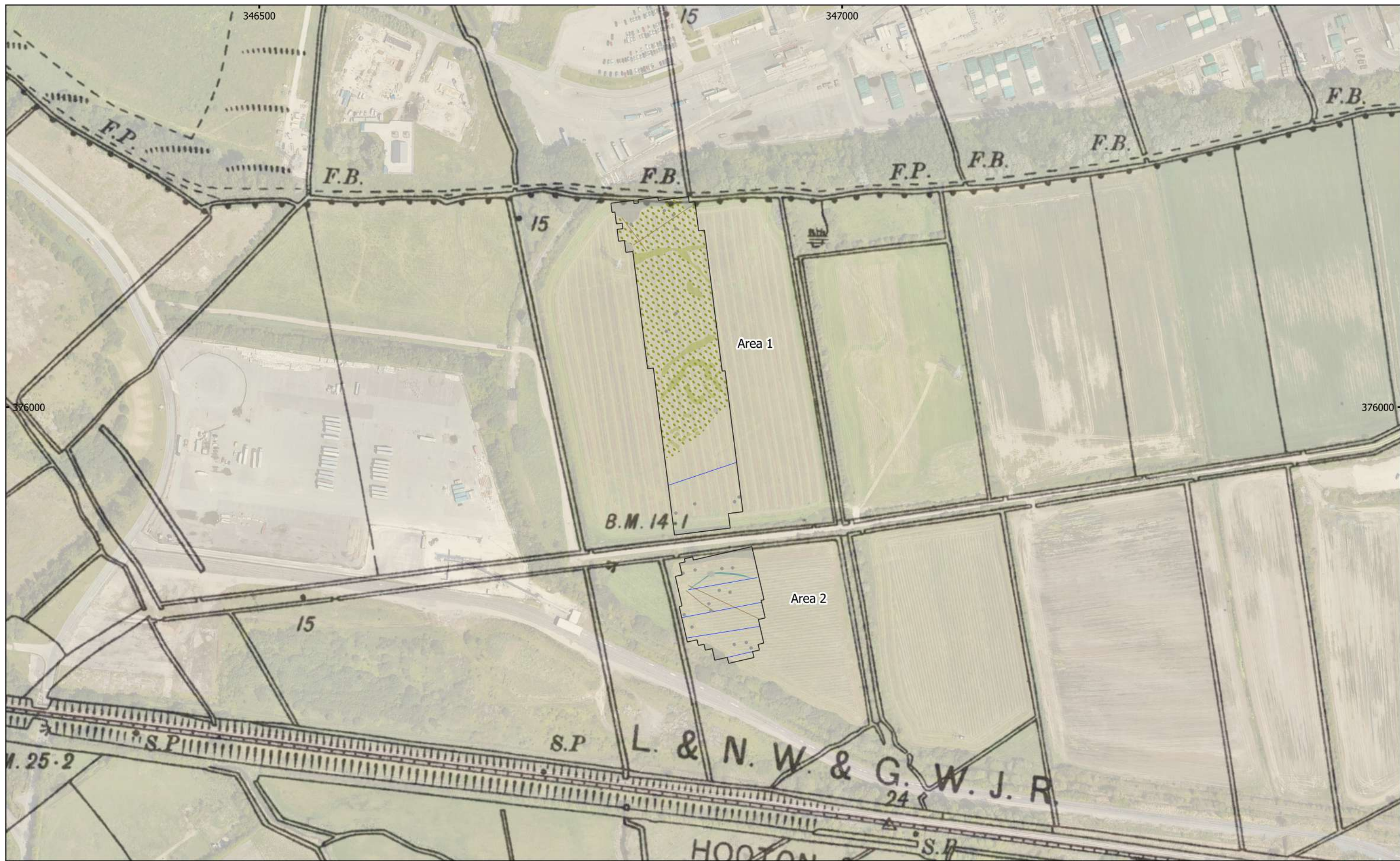
MSSJ1172 - HyNet CO2 Pipeline Figure 59 - Magnetic Interpretation Over Historical Maps (Overview) (Areas 1 & 2) 1:3,000 @ A3 Copyright Magnitude Surveys Ltd 2022 Contains historical mapping © CLS Data 2022: Ordnance Survey, 6" 2nd edition c. 1882-1913
