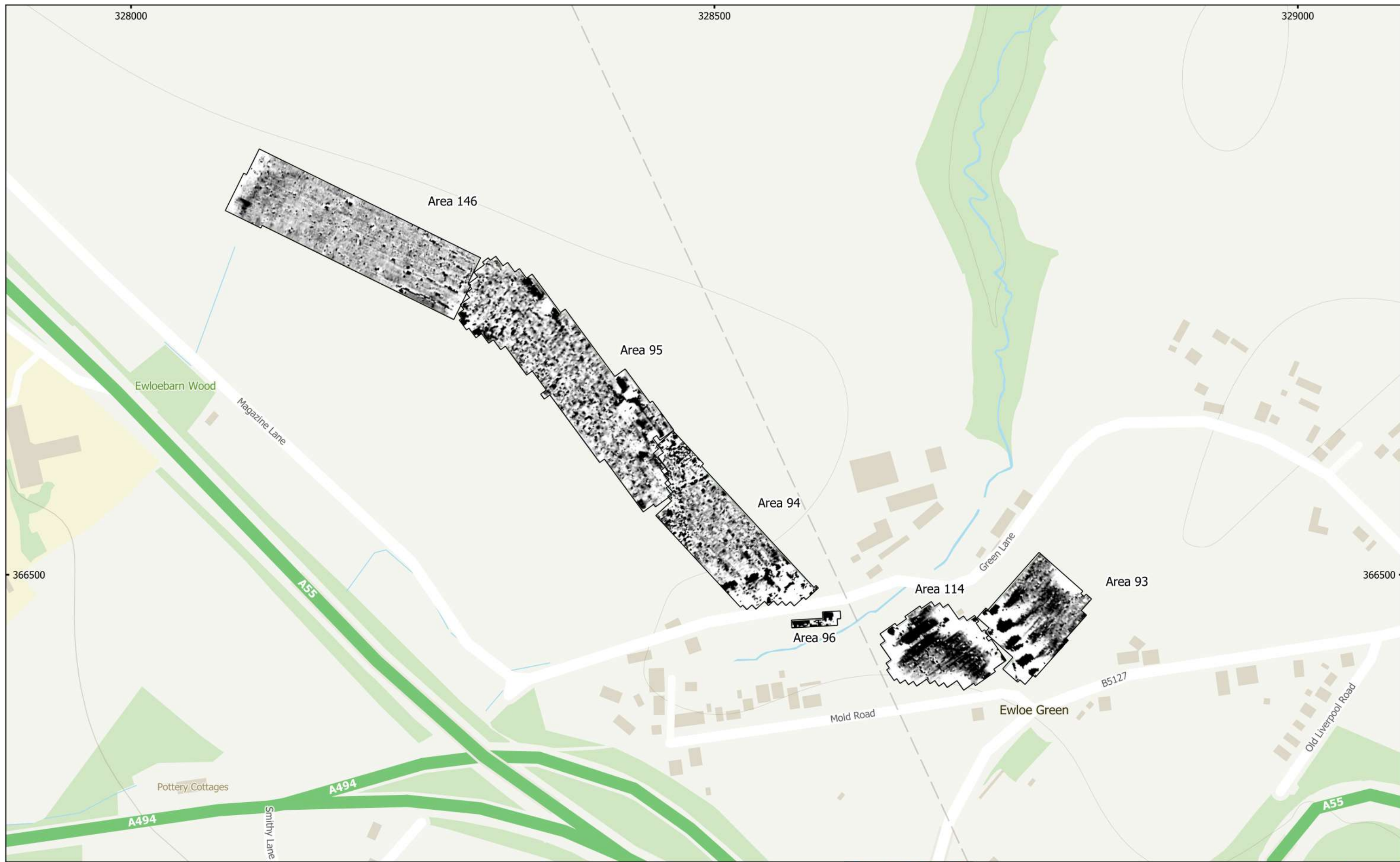
MSSJ1172 - HyNet CO2 Pipeline Figure 16 - Magnetic Total Field (Lower Sensor) (Overview) (Areas 146, 95, 94, 96, 114, & 93) 1:3,000 @ A3 Copyright Magnitude Surveys Ltd 2022 Contains Ordnance Survey data © Crown Copyright and database right 2022
