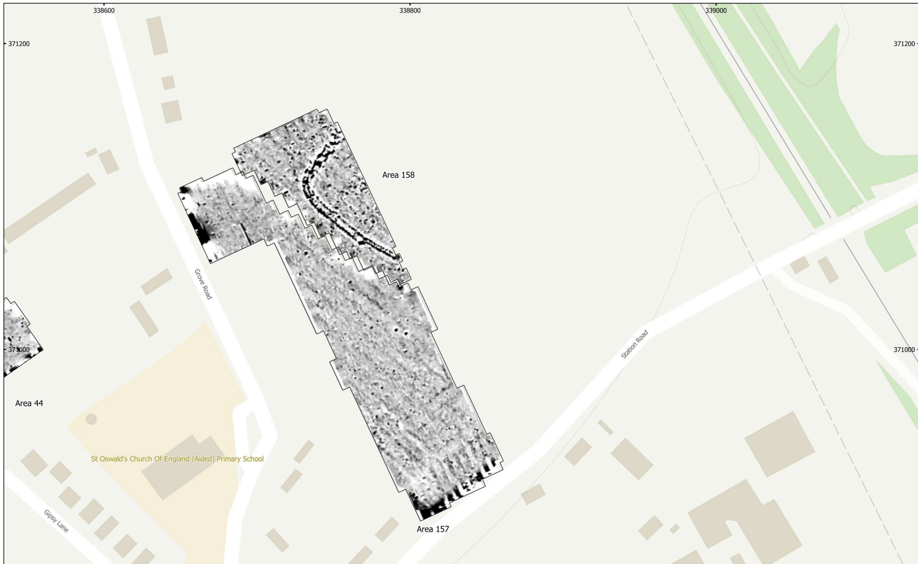
MSSJ1172 - HyNet CO2 Pipeline Figure 171 - Magnetic Gradient (Areas 44, 157 & 158) 1:1,500 @ A3 Copyright Magnitude Surveys Ltd 2022 Contains Ordnance Survey data © Crown Copyright and database right 2022
