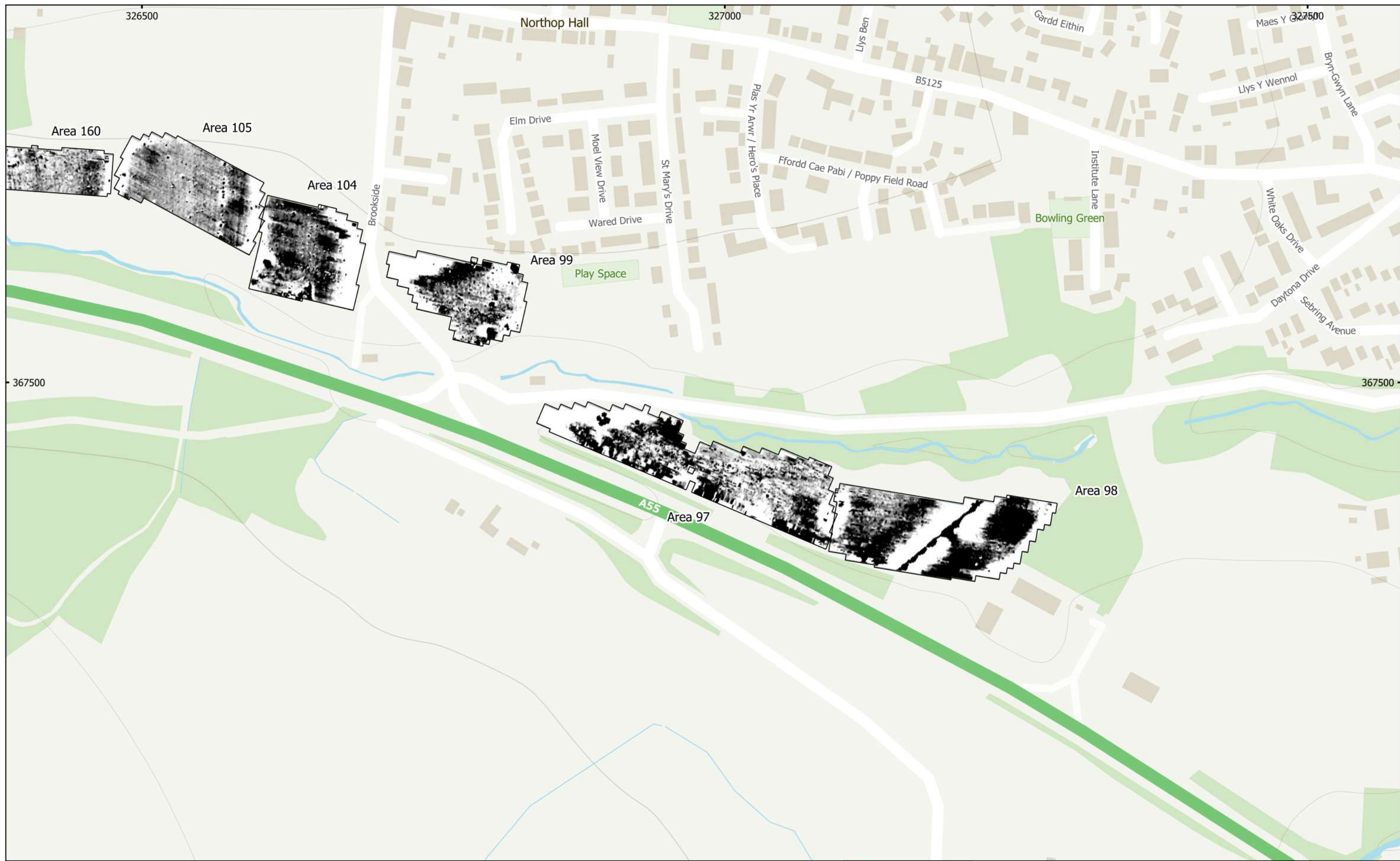
MSSJ1172 - HyNet CO2 Pipeline Figure 14 - Magnetic Total Field (Lower Sensor) (Overview) (Areas 160, 105, 104, 99, 97, & 98) 1:3,000 @ A3 Copyright Magnitude Surveys Ltd 2022 Contains Ordnance Survey data © Crown Copyright and database right 2022
