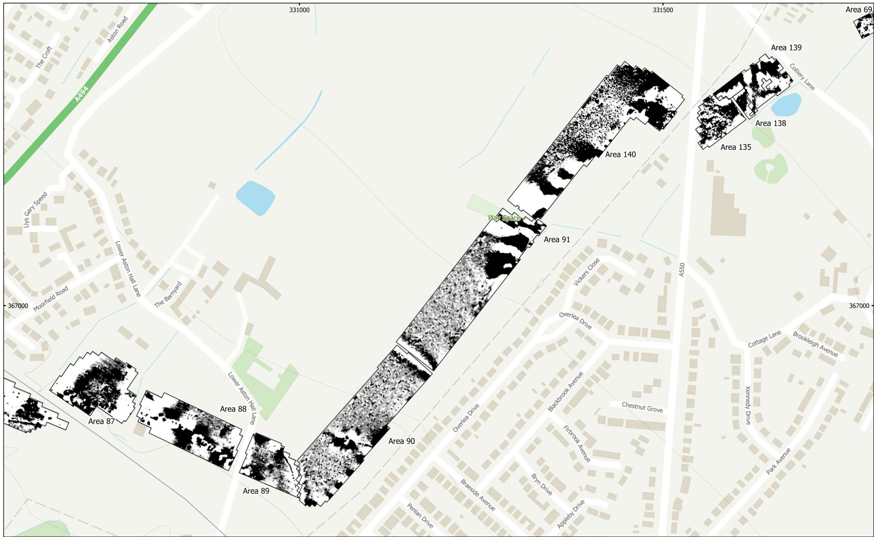
MSSJ1172 - HyNet CO2 Pipeline Figure 20 - Magnetic Total Field (Lower Sensor) (Overview) (Areas 85, 87, 88, 89, 90, 91, 140, 135, 138, & 139) 1:3,000 @ A3 Copyright Magnitude Surveys Ltd 2022 Contains Ordnance Survey data © Crown Copyright and database right 2022
