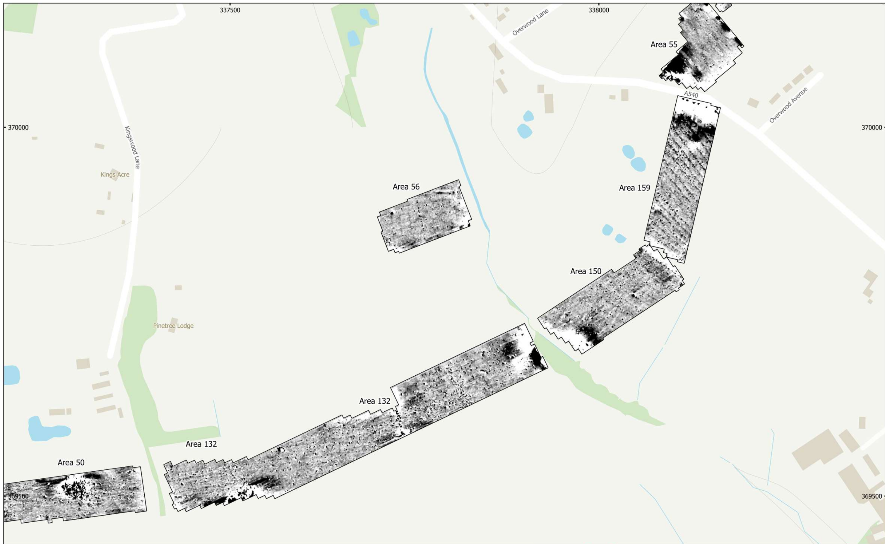
MSSJ1172 - HyNet CO2 Pipeline Figure 34 - Magnetic Total Field (Lower Sensor) (Overview) (Areas 50, 132, 56, 150, 159, & 55) 1:3,000 @ A3 Copyright Magnitude Surveys Ltd 2022 Contains Ordnance Survey data © Crown Copyright and database right 2022
