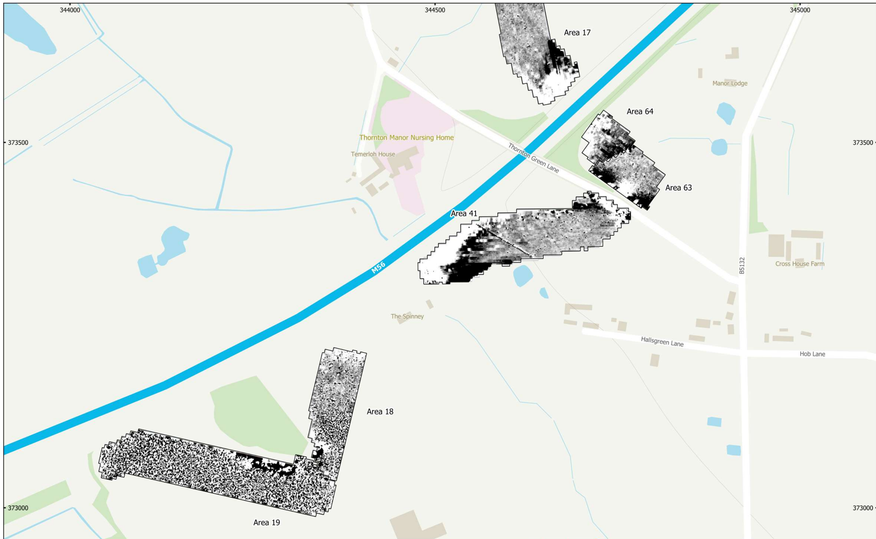
MSSJ1172 - HyNet CO2 Pipeline Figure 48 - Magnetic Total Field (Lower Sensor) (Overview) (Areas 19, 18, 41, 63, 64, & 17) 1:3,000 @ A3 Copyright Magnitude Surveys Ltd 2022 Contains Ordnance Survey data © Crown Copyright and database right 2022
