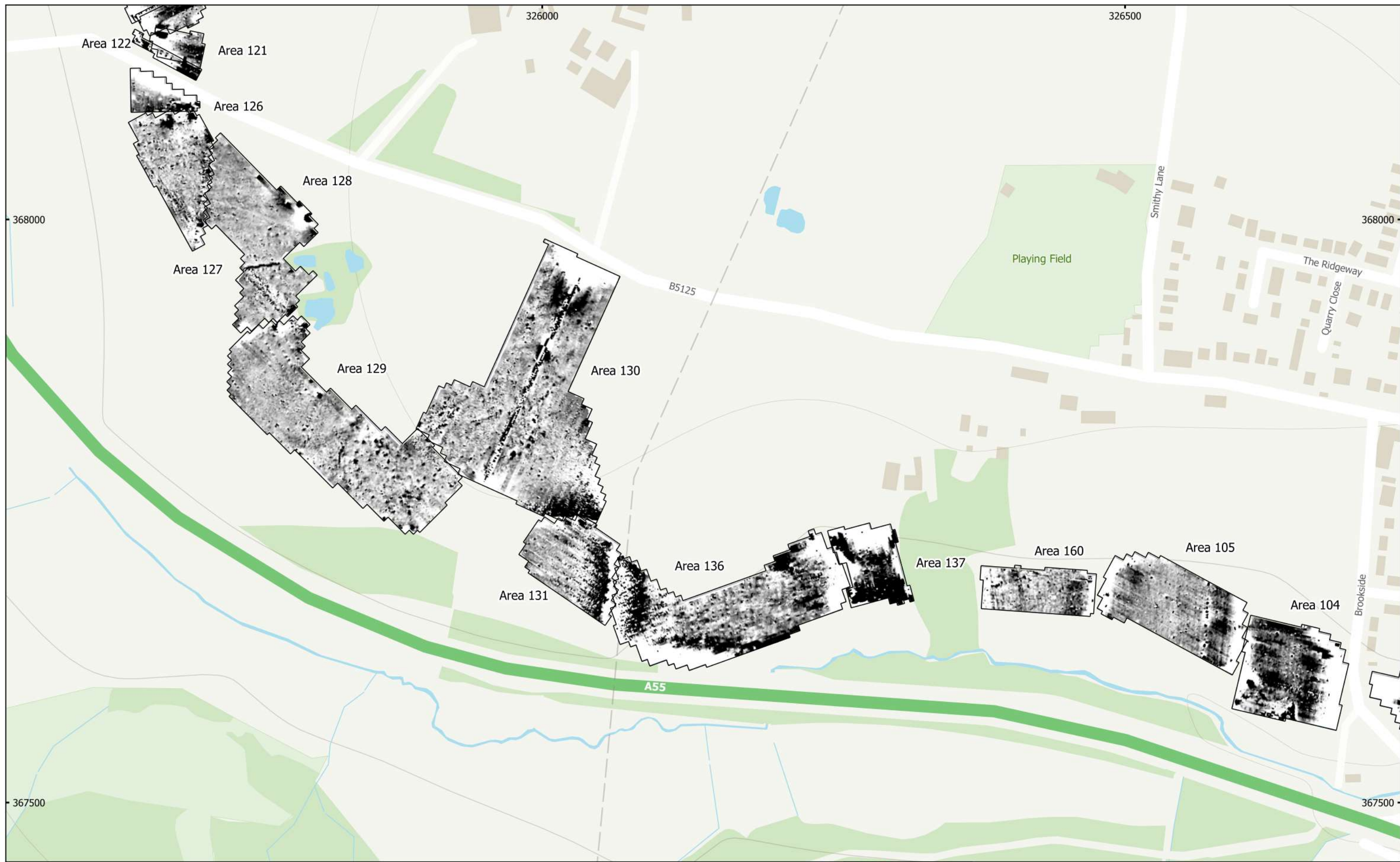
MSSJ1172 - HyNet CO2 Pipeline Figure 12 - Magnetic Total Field (Lower Sensor) (Overview) (Areas 120, 122, 121, 126, 128, 127, 129, 130, 131, 136, 137, 160, 105, & 104) 1:3,000 @ A3 Copyright Magnitude Surveys Ltd 2022 Contains Ordnance Survey data © Crown Copyright and database right 2022
