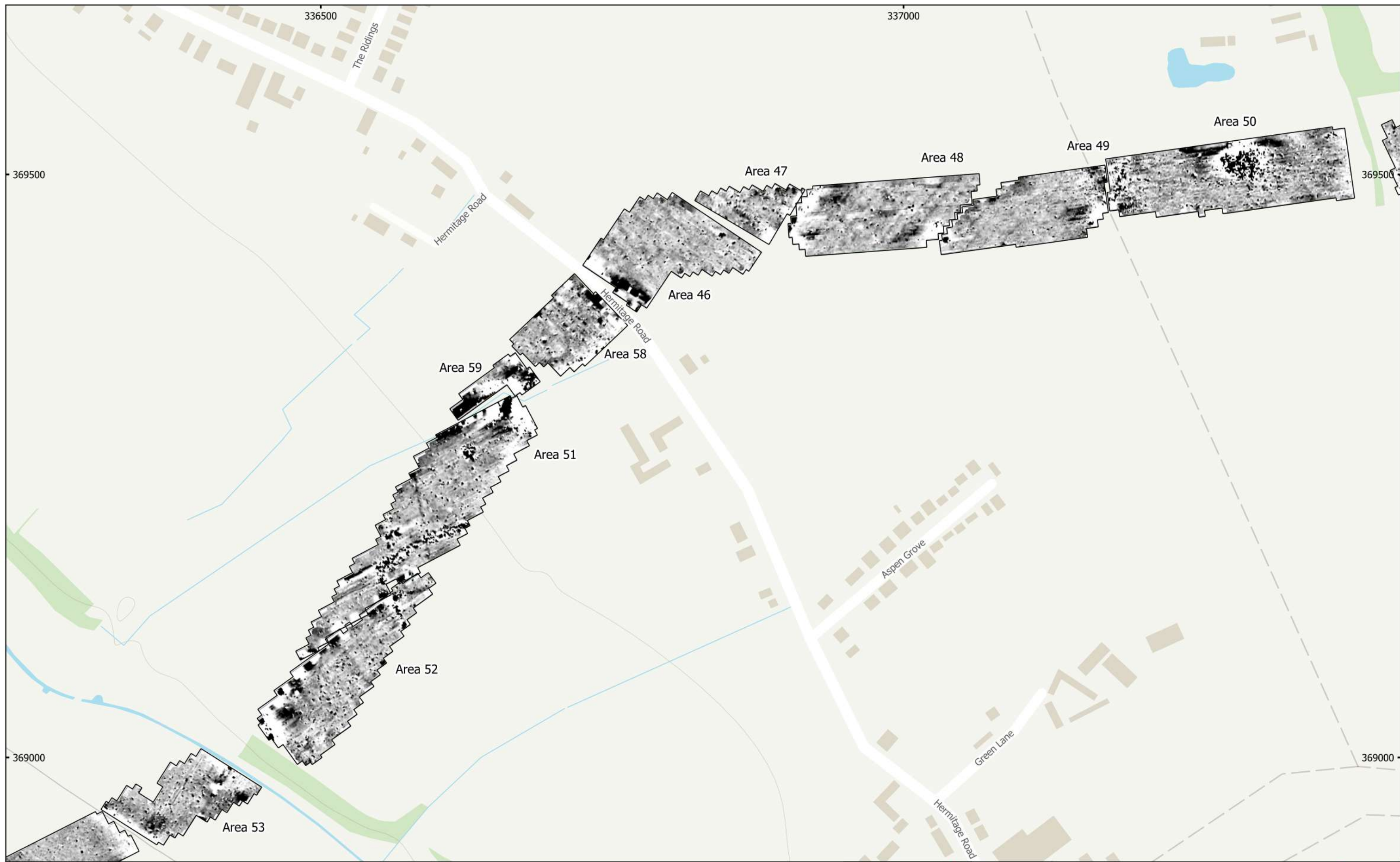
MSSJ1172 - HyNet CO2 Pipeline Figure 32 - Magnetic Total Field (Lower Sensor) (Overview) (Areas 53, 52, 51, 59, 58, 46, 47, 48, 49, & 50) 1:3,000 @ A3 Copyright Magnitude Surveys Ltd 2022 Contains Ordnance Survey data © Crown Copyright and database right 2022
