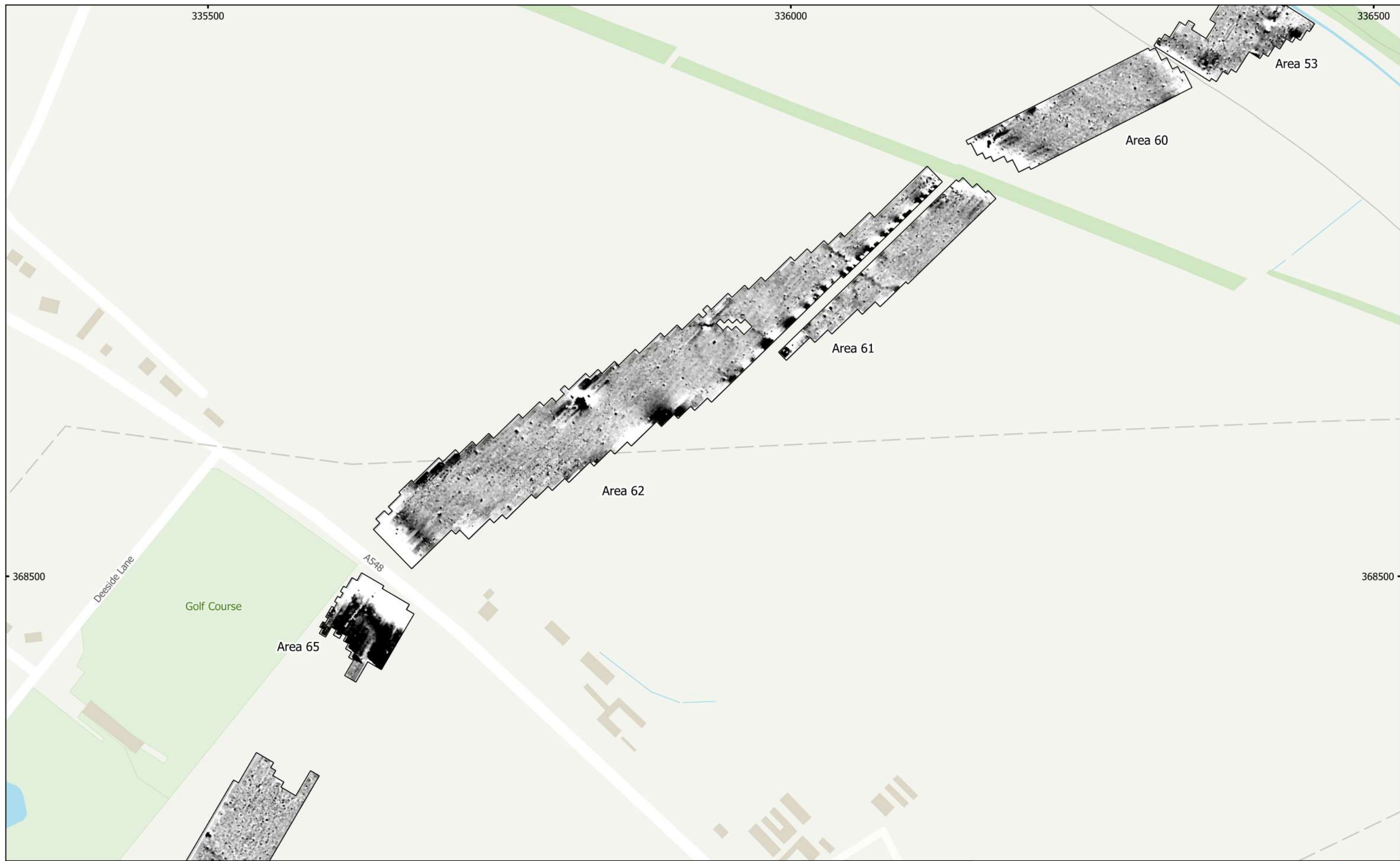
MSSJ1172 - HyNet CO2 Pipeline Figure 30 - Magnetic Total Field (Lower Sensor) (Overview) (Areas 65, 62, 61, 60, & 53) 1:3,000 @ A3 Copyright Magnitude Surveys Ltd 2022 Contains Ordnance Survey data © Crown Copyright and database right 2022
