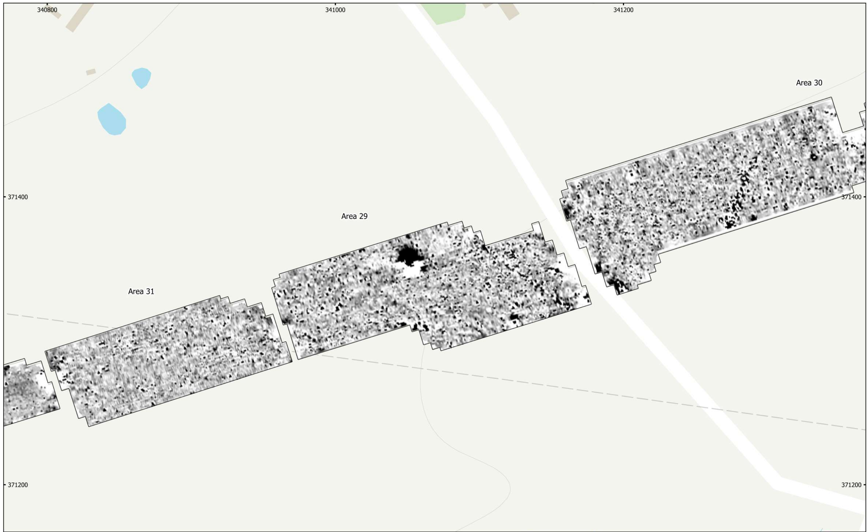
MSSJ1172 - HyNet CO2 Pipeline Figure 183 - Magnetic Gradient (Areas 31, 29, & 30) 1:1,500 @ A3 Copyright Magnitude Surveys Ltd 2022 Contains Ordnance Survey data © Crown Copyright and database right 2022
