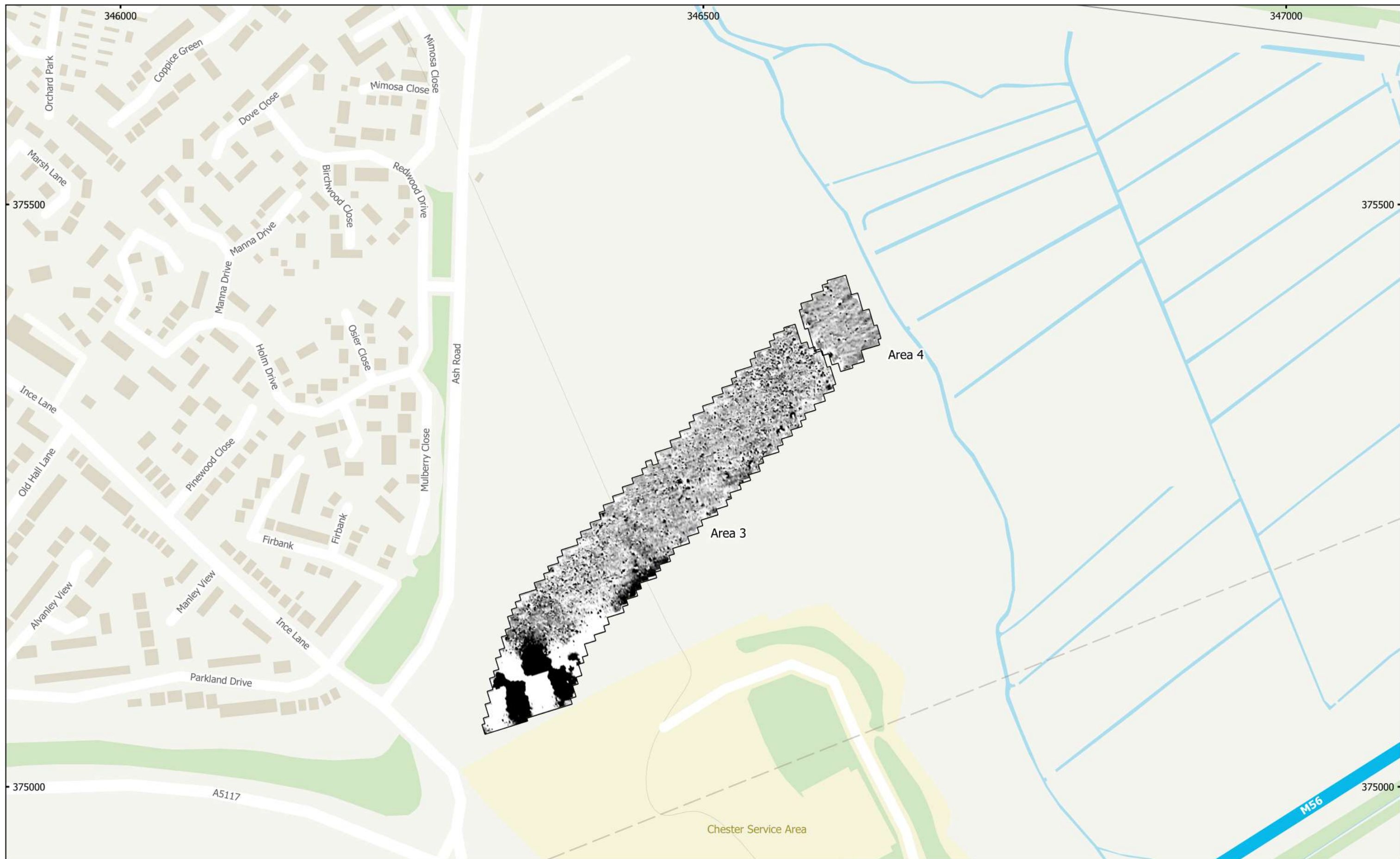
MSSJ1172 - HyNet CO2 Pipeline Figure 56 - Magnetic Total Field (Lower Sensor) (Overview) (Areas 3 & 4) 1:3,000 @ A3 Copyright Magnitude Surveys Ltd 2022 Contains Ordnance Survey data © Crown Copyright and database right 2022
