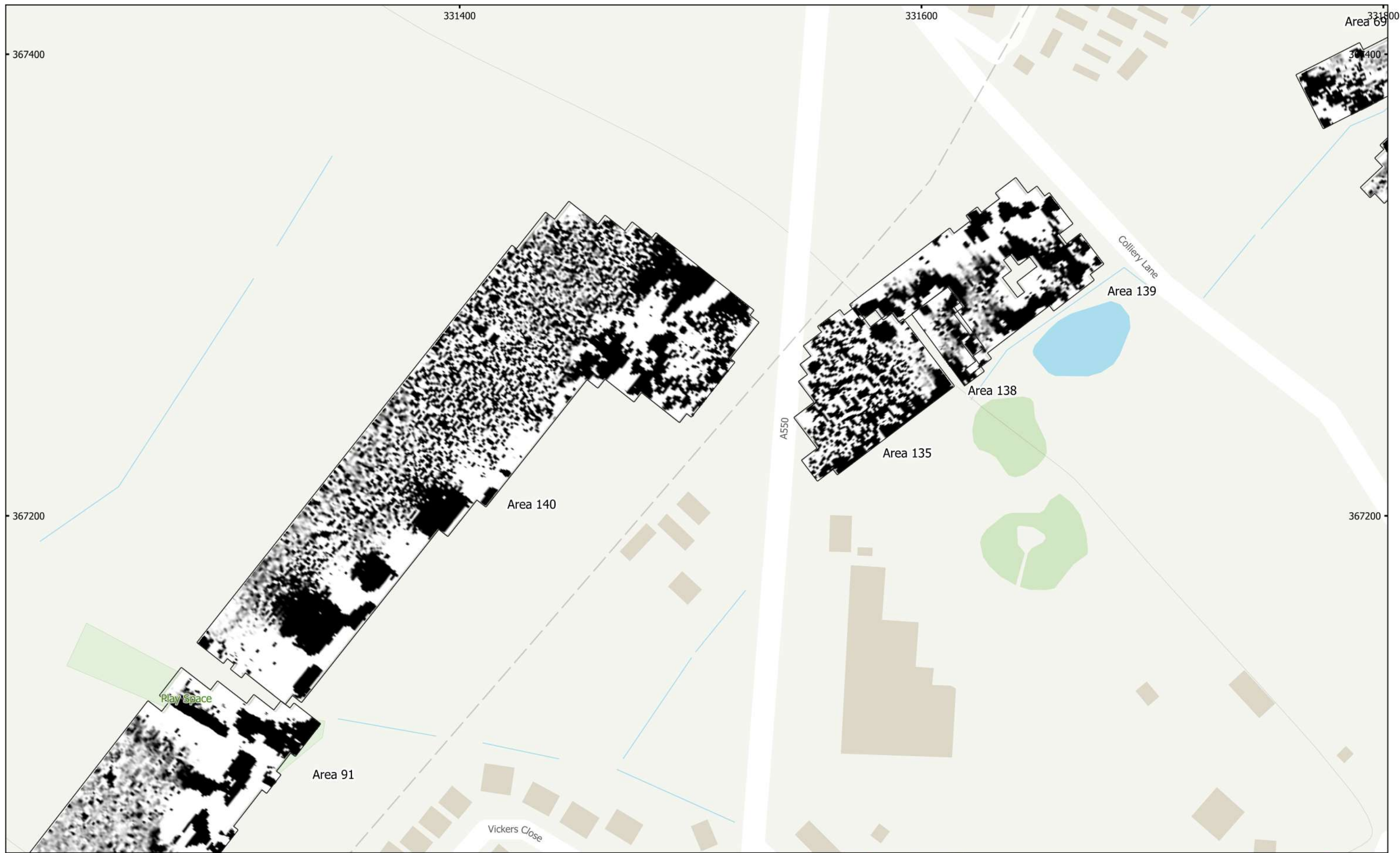
MSSJ1172 - HyNet CO2 Pipeline Figure 114 - Magnetic Gradient (Areas 68, 69, 91, 135, 138, 139 & 140) 1:1,500 @ A3 Copyright Magnitude Surveys Ltd 2022 Contains Ordnance Survey data © Crown Copyright and database right 2022
