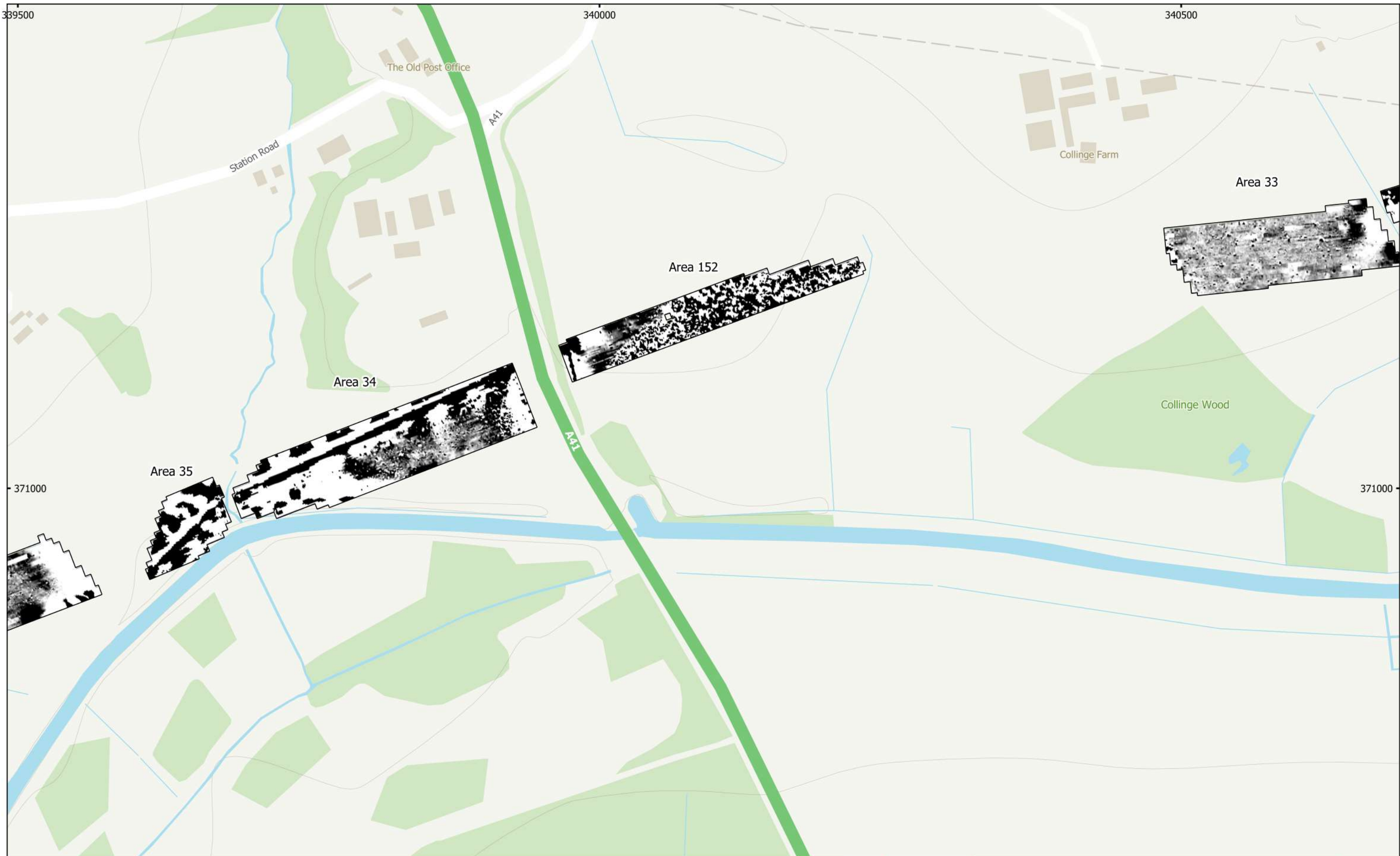
MSSJ1172 - HyNet CO2 Pipeline Figure 40 - Magnetic Total Field (Lower Sensor) (Overview) (Areas 36, 35, 34, 152, & 33) 1:3,000 @ A3 Copyright Magnitude Surveys Ltd 2022 Contains Ordnance Survey data © Crown Copyright and database right 2022
